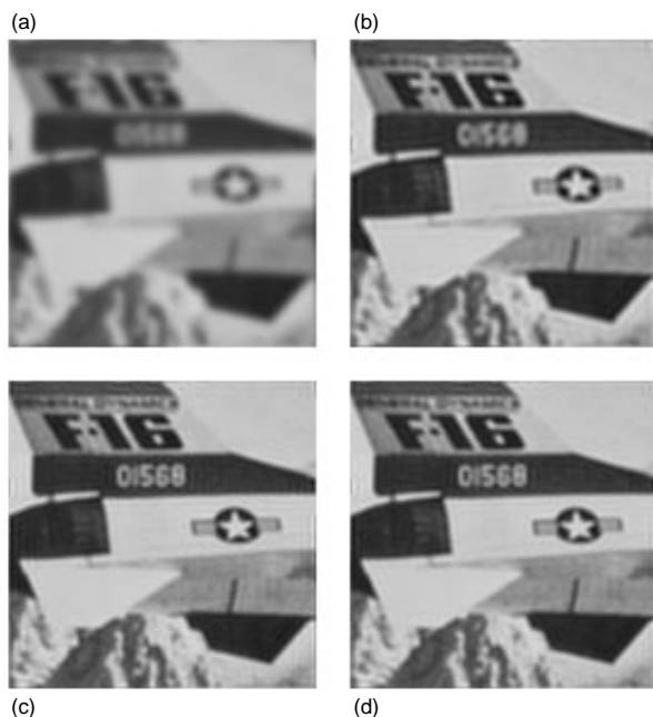
Figure 4: Blurred and restored images using R–L; (a) blurred, (b) unaccelerated RL0(250), (c) accelerated RL1(250), (d) unaccelerated RL0(10,000).
